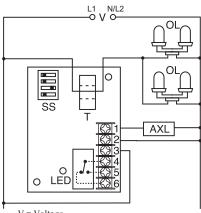
V = Voltage OL = Obstruction Lamps T = Toroid SS = Selector Switch AXL = Auxiliary Load/Alarm Relay contacts are isolated.
